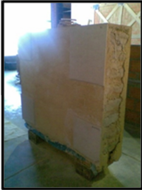
Fig. 2. Application of mortars on adobe wall.
